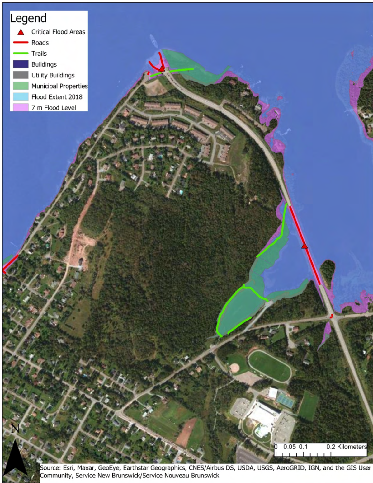
Figure 18: Critical flood locations displaying historical flooding (5.73m) and projected flooding for 2100 (7m) at Gondola Point, Quispamsis, NB (2018) (Daigle, 2020).
