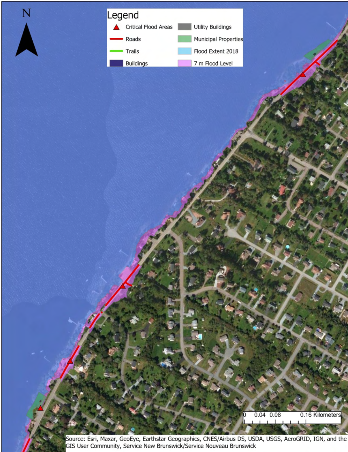
Figure 19: Critical flood locations displaying historical flooding (5.73m) and projected flooding for 2100 (7m) on Gondola Point Road from 623 Gondola Point Road to 565 Gondola Point Road (Daigle, 2020).
